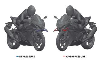
Due to its angles and frontal surface, it creates an overpressure on the top of the spoiler. The turbulance create below, generates a difference of pressure between the upper and lower part of the spoiler. Which ultimately generates the aerodynamic downforce.
